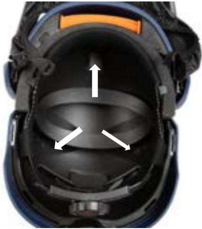
**10.1** Remove the head harness from the helmet by releasing the three fixing points.
