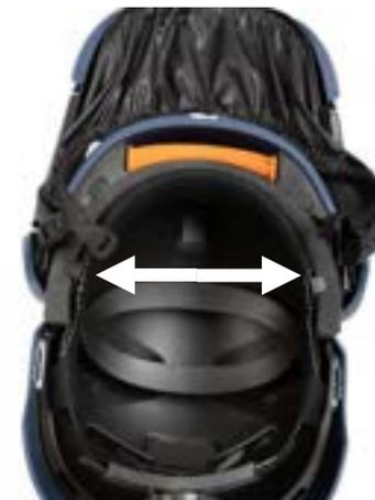
**8.4** Place the seal so it fits between the sockets of the sides of the head harness. Check that head harness seal is mounted as shown.
